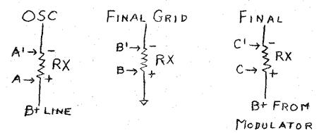
ADD RX'S IN SERIES WITH EXISTING CIRCUITS (RX'S- 1W-5% RESISTORS ONLY FOR ACCURACY)
