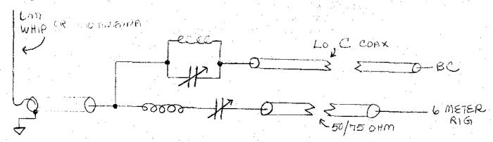
L1 & C1 form a series 6 meter tuned circuit whose impedence is low at 6m and high at BC frequencies. It then passes the 6 m info and blocks the BC signals.
