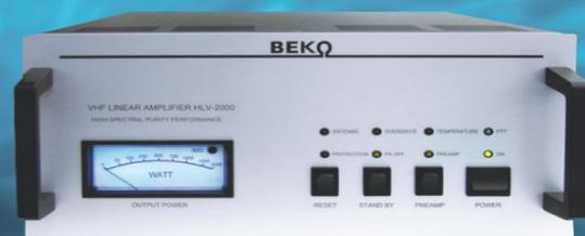
**Instant ON • Built-In Preamp Sequencer • Overdrive...Temp. & VSWR Protected**
